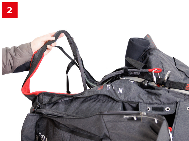
Route the rescue bridles through the zip bridle tunnel. And close the zipper until the end
