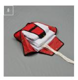
Place the folded rescue into the inner bag. Fold 60cm of line under the rescue.
